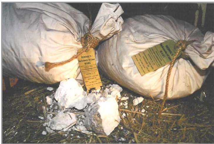
Marl is a crumbly, off-white substance.
